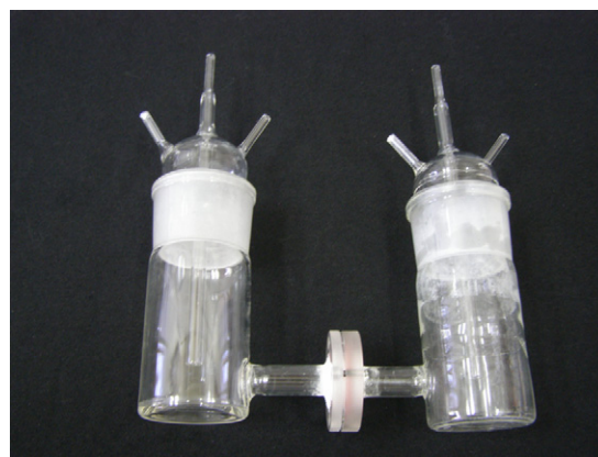
Fig. 9. Photograph of a convenient laboratory PEC H-shaped reactor made of pyrex glass. Ion-transport membrane is supported in the middle. Fittings with tubing allow electrode connections and gas inlet–outlet.
